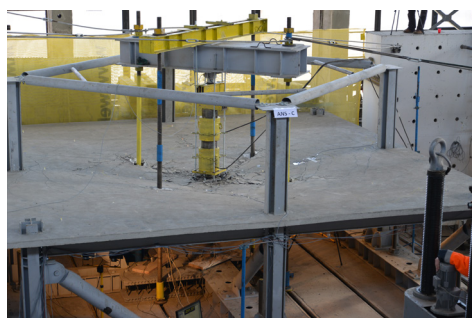
Fig. 5. Experimental test on 3D composite frame system
